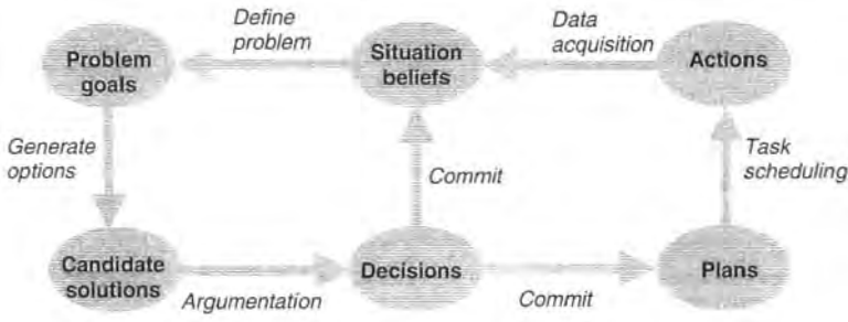
Figure 17-2. The generalized domino model of Fox and Das (2000). The ellipses refer to states of the system (representations), the arrows are processes (J. Fox, personal communication).
